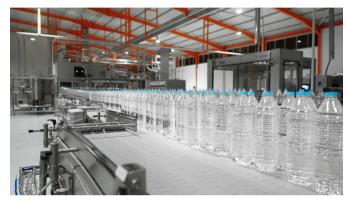
As one of the leading bottled water producers in Iraq, Durrat Al Khaleej aims to provide the best experience to consumers. Sidel's packaging solutions successfully fulfilled its goal by delivering a complete water line with a lightweighted and simultaneously stable PET bottle design, weighing only 10.5 grams for the 500 ml bottle format, at a time of very high travel restrictions in Iraq.
